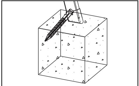
Set the stakes in concrete (as shown).
